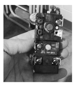
Recently we discovered a charred electric water heater thermostat - it had caught fire due to faulty electrical connections.
